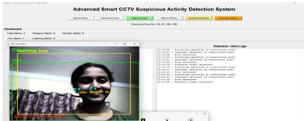
Figure 5 Intruder and loitering detection in restricted zone
